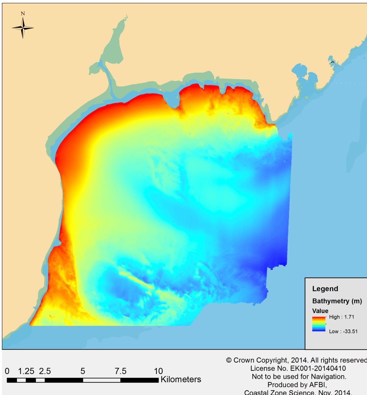
Figure 3.1. Multibeam bathymetry for Dundrum Bay.
