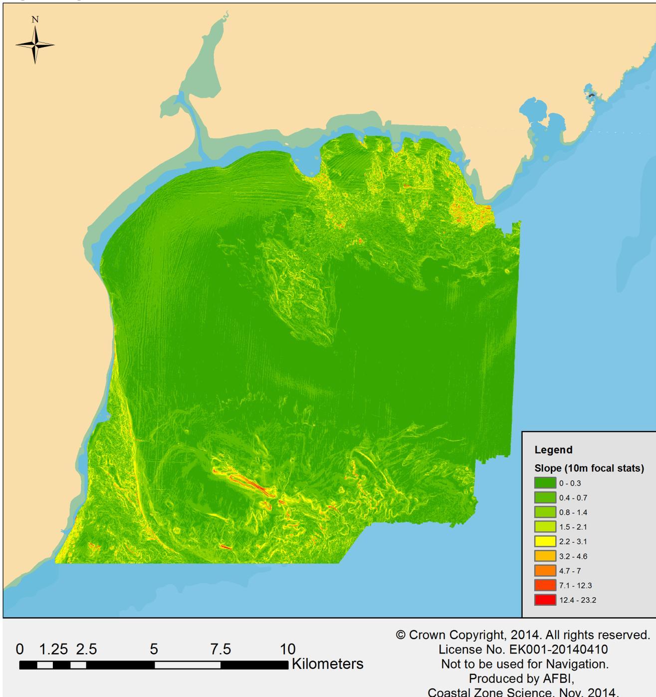
Figure 3.3. Slope angles (in degrees) for Dundrum Bay.
