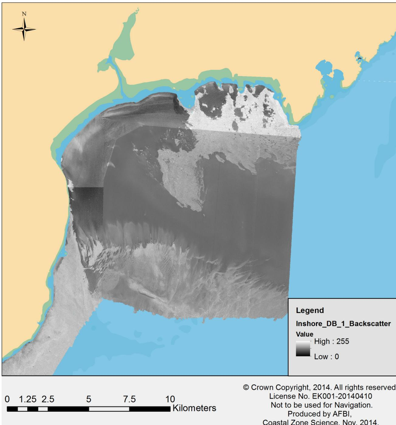
Figure 3.3 Multibeam backscatter mosaics for Dundrum Bay. Low image values = low reflectivity (softer ground), high image values = high reflectivity (harder or rougher ground).
