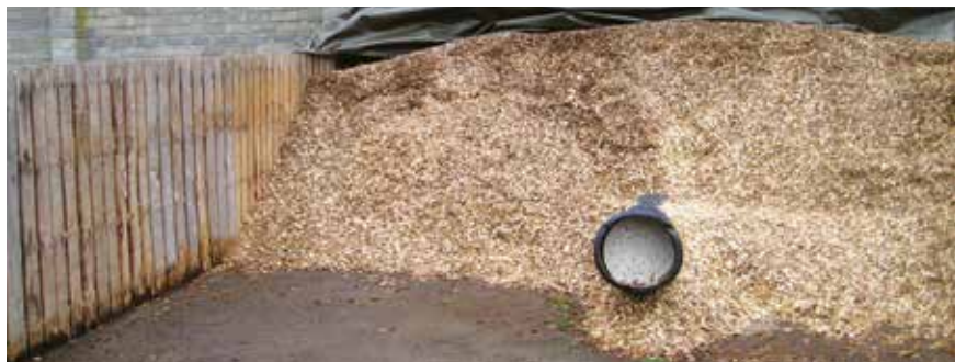
Farmyard clamp for drying willow chips
