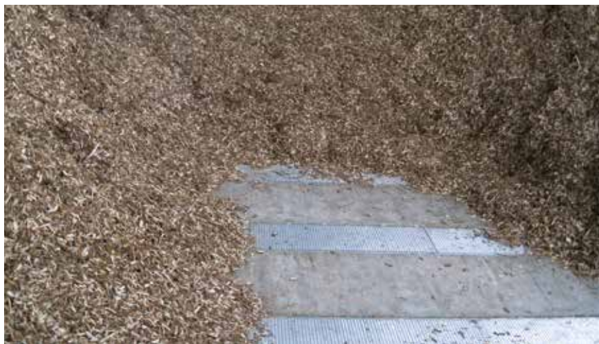
Willow chip is dried from +50% moisture at harvest to less than 30% moisture to prevent dry matter losses through biological composting and physical degradation of the willow chip
