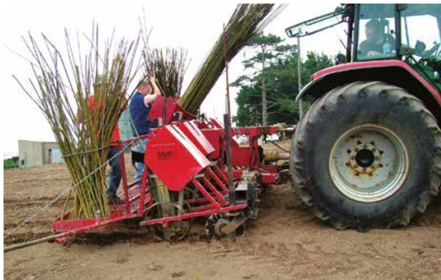
Planting using a Step planter - when completed the site should be rolled to consolidate the surface
