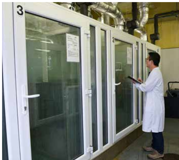
Figure 1. AFBI Cattle Respiration Calorimeter Unit
