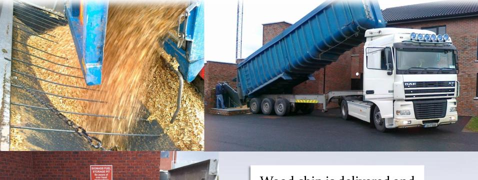
Wood chip is delivered and conveyed to the users fuel store, by means appropriate to the site and user needs.
