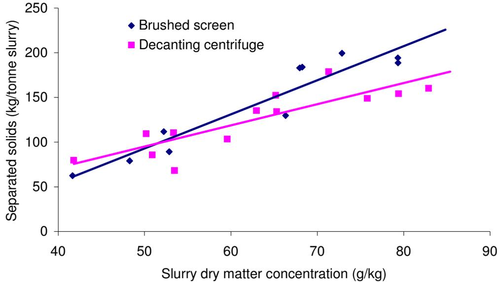
**Figure 11.** Relationship between cattle slurry dry matter concentration and the weight of fresh solids produced from 1 tonne of cattle slurry without chemicals.
