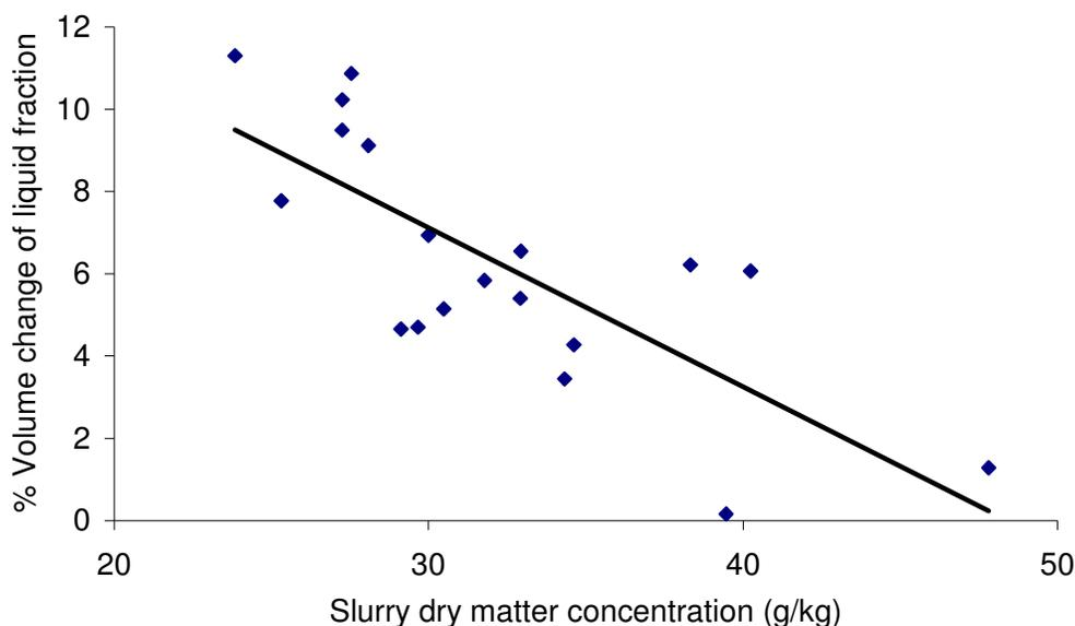
**Figure 7.** Relationship between pig slurry dry matter concentration and percentage volume change in supernatant, relative to the slurry volume, for the chemical treatments in the decanting centrifuge.
