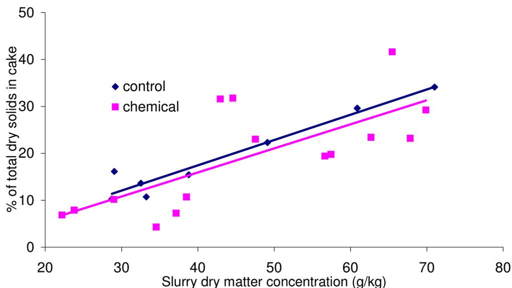
**Figure 4.** Brushed Screen: Relationship between pig slurry dry matter concentration and percentage of dry solids partitioned to the separated solid fraction.
