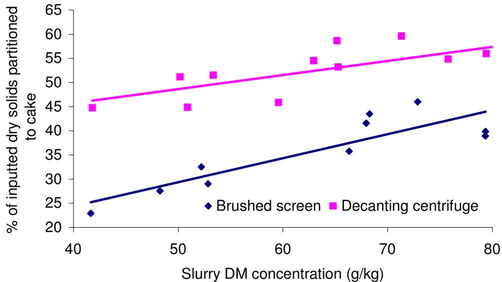
**Figure 12.** Relationship between cattle slurry dry matter concentration and the percentage of inputted dry solids partitioned to the separated solids fraction for the control treatments in the decanting centrifuge and brushed screen separator.
