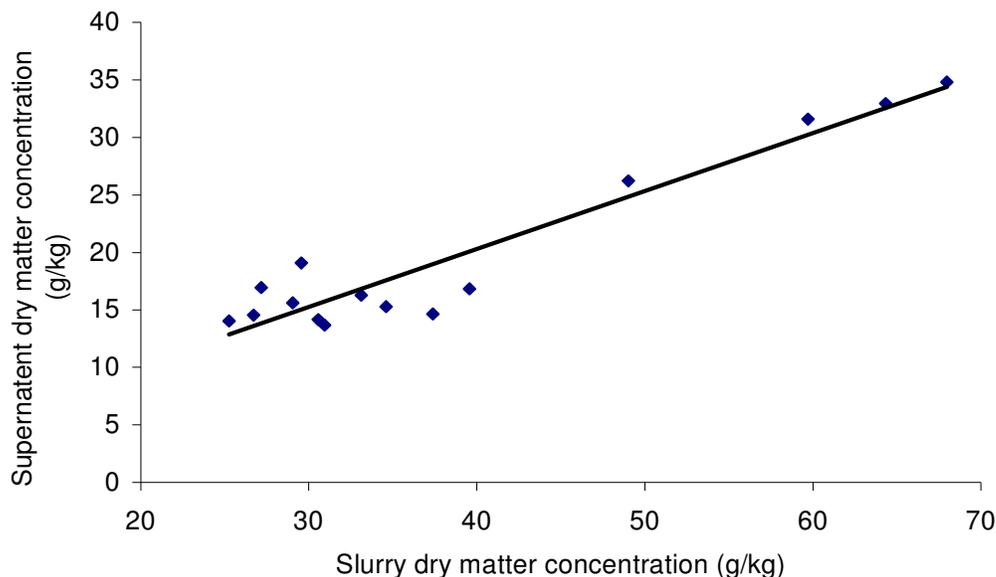
**Figure 5.** Relationship between pig slurry dry matter concentration and supernatant dry matter concentration for the decanting centrifuge, without chemical addition.
