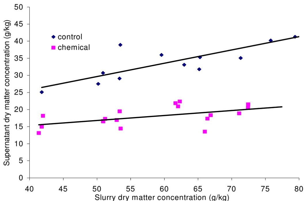
**Figure 10.** Relationship between cattle slurry dry matter concentration and supernatant dry matter concentration, for cattle slurry separated through a decanting centrifuge.
