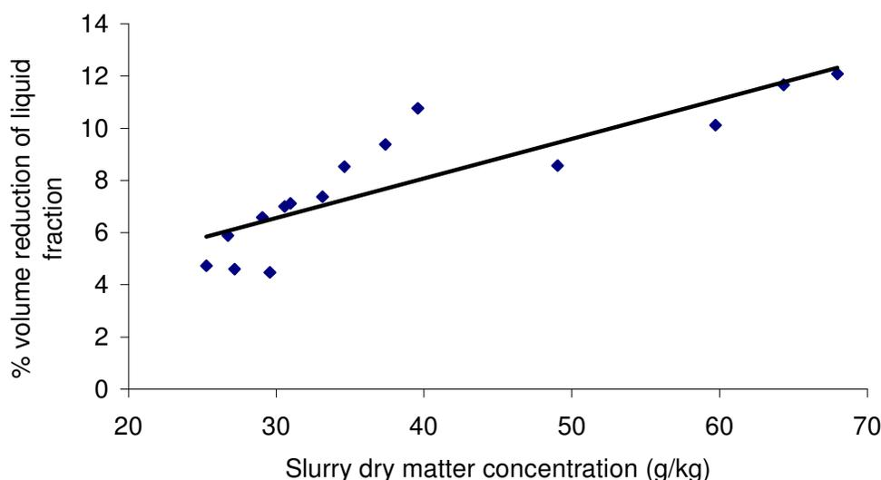
**Figure 6.** Relationship between percentage volume reduction of supernatant (relative to slurry input volume) and slurry dry matter concentration for the control treatments with the decanting centrifuge.
