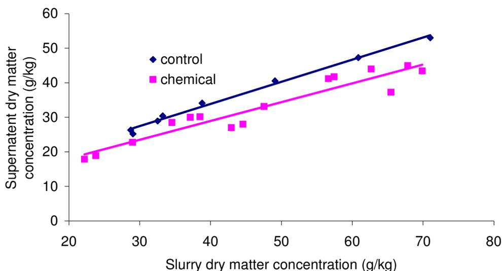
**Figure 3.** Brushed screen: Relationship between pig slurry dry matter concentration and supernatant dry matter concentration.
