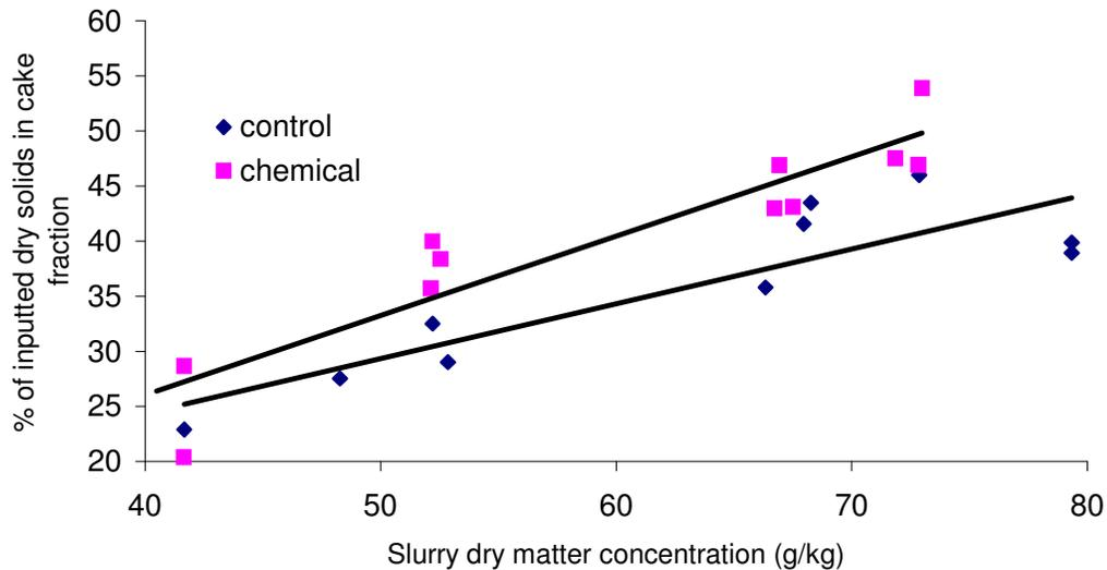
**Figure 9.** Relationship between cattle slurry dry matter concentration and the percentage of dry solids partitioned to the separated solid fraction with the brushed screen separator.
