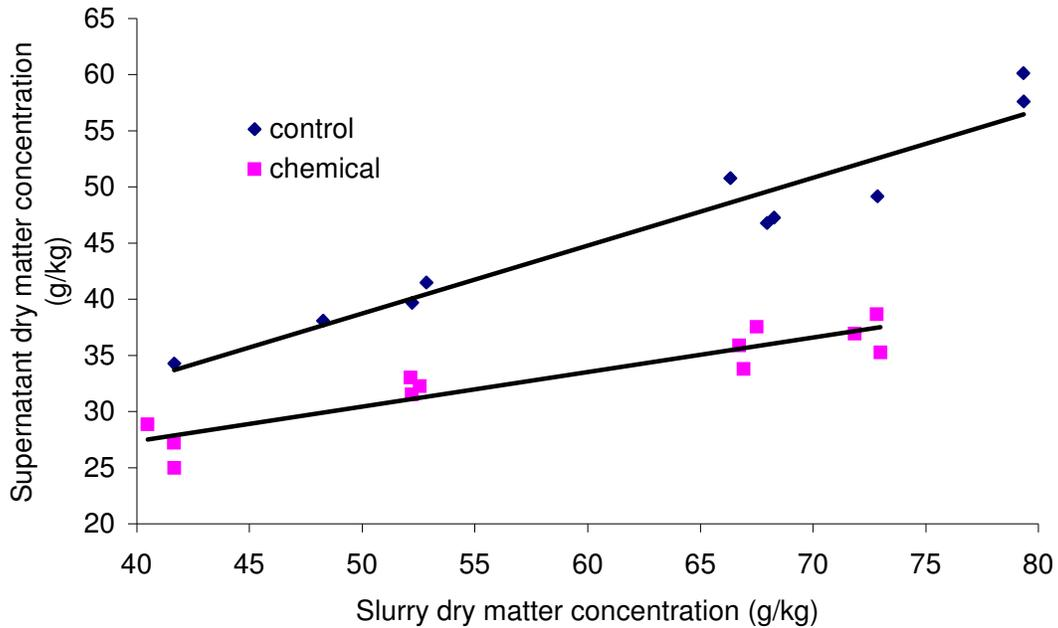
**Figure 8.** Relationship between cattle slurry dry matter concentration and supernatant dry matter concentration for the brushed screen separator.
