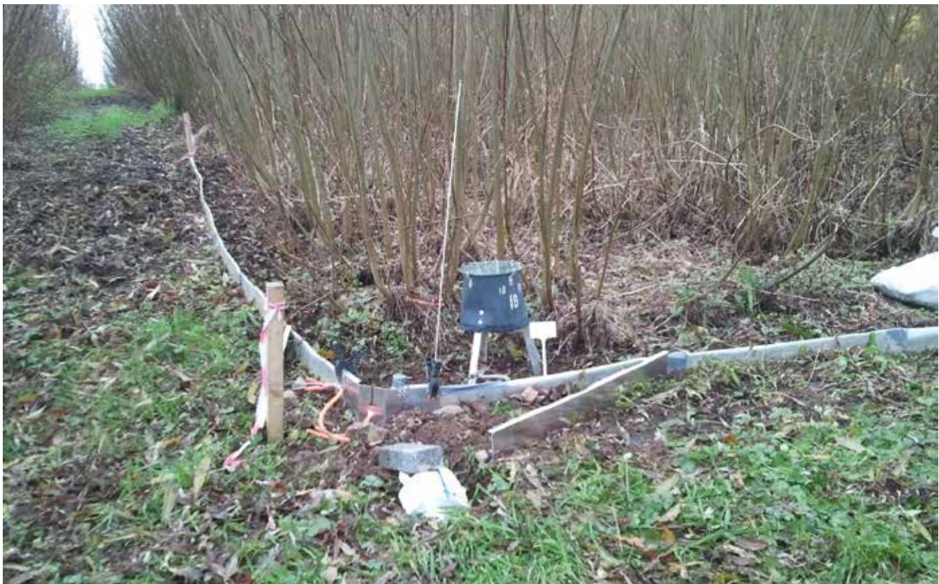
Overland flow measuring point including weir and datalogger. The volume, as well as the time and duration of overland flow are recorded.
