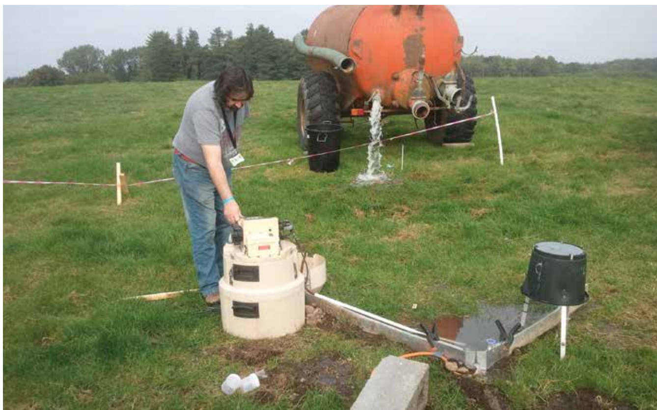
Calibration of overland flow weirs
