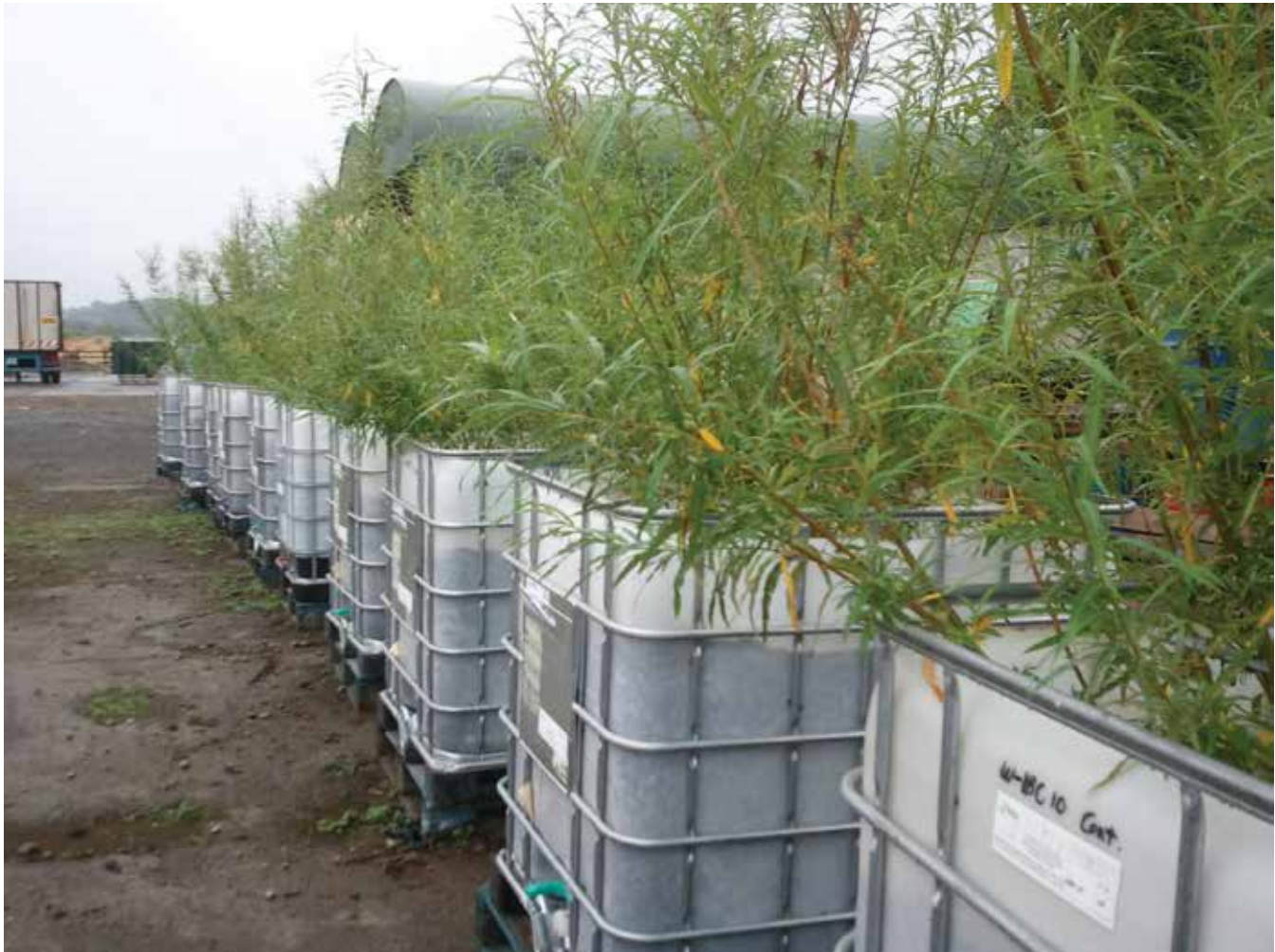
Large scale lysimeters planted with willow being used to measure overland flow and leaching
